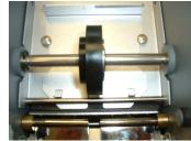
2. Wash out the moistening brushes in soap or mild detergent and place both brushes into the tank so the angle on the brushes slopes towards the rear of the tank (see figure # 3). Insert the tank into the opening in front of the machine being sure the tank is behind the upward lip on the tank shelf.
